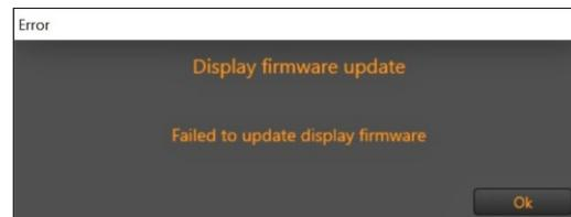
If this error occurred before re-starting the device, HFD will not show a warning but the IR-receiver is unresponsive and the display is still showing bootloader-mode.
